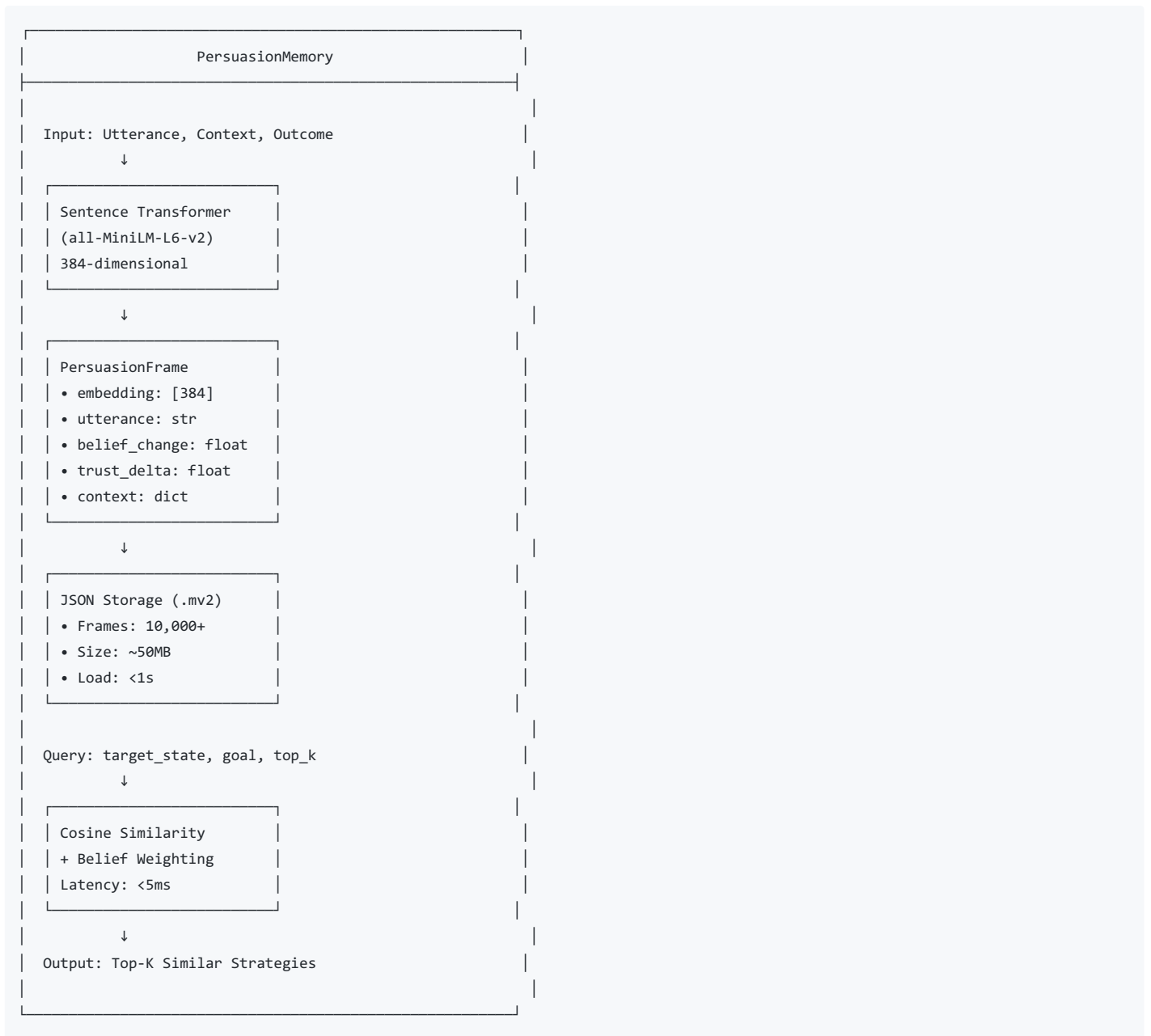
Figure 3: Memory architecture with MemVid integration
