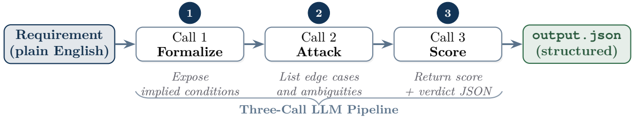
Figure 1. The three-stage pipeline. Each GST requirement is first formalized into explicit bullet-point rules, then audited for edge cases, and finally scored as structured JSON. All calls use fixed system prompts.
